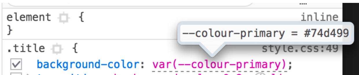
Figure 4: Screenshot of the devtools in Firefox, inspecting a variable
